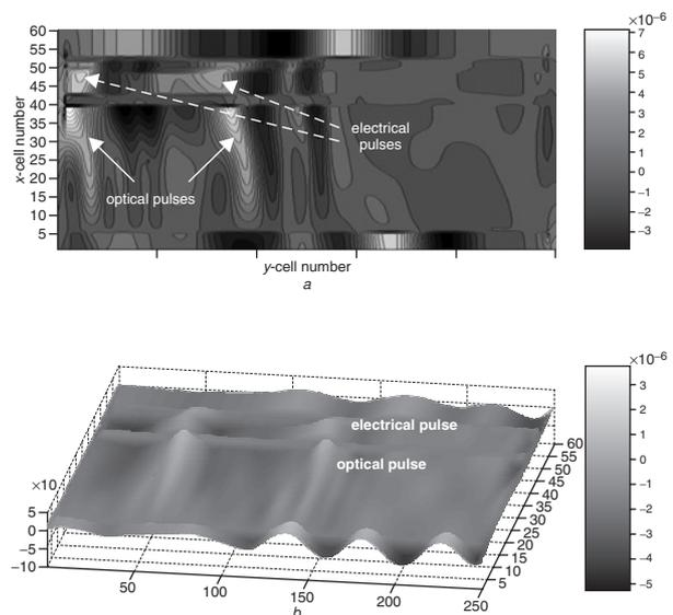
**Fig. 2** Snapshots of  $E_x$ -field spatial distribution at the  $z = 51$  plane at two time steps
