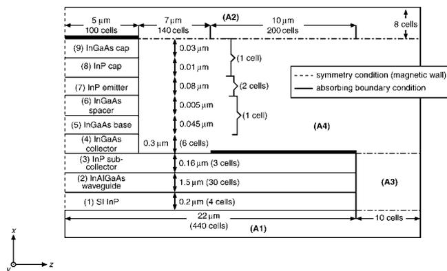
**Fig. 1** Cross-section of TW-HPT used in FDTD simulation
