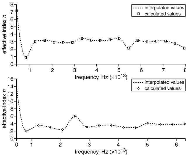
**Fig. 3** Effective refractive indices of optical and electrical wave
