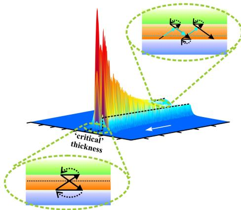
**Figure 2.** Snapshot of the propagation of a monochromatic light signal along the negative-index heterostructure. The lightwave completely stops upon reaching the 'critical' thickness. The top right and bottom left insets associate the wave propagation with the corresponding zigzag ray analysis for the corresponding guide widths.
