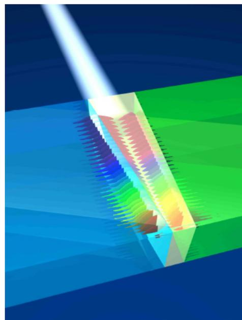
**Figure 1.** A white light beam hits the tapered negative refractive index layer (shown in white), which is surrounded by two regular dielectric layers (shown in blue and green). Upon entering the structure, each frequency component, or color, of the beam stops at different thicknesses, forming a trapped rainbow.
